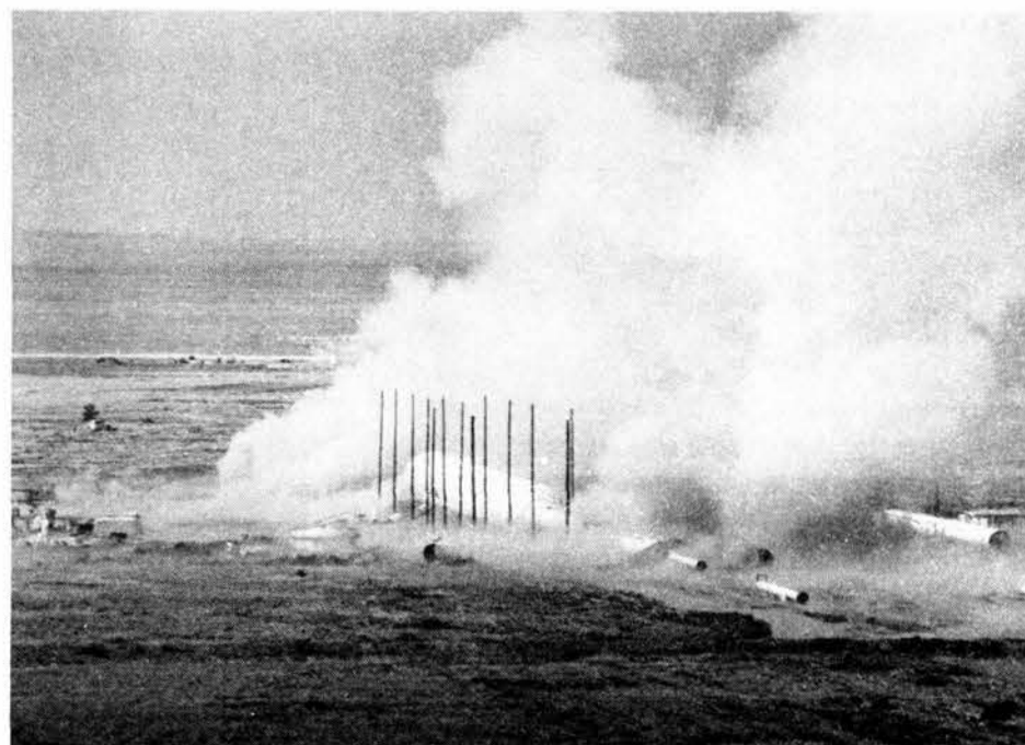
nuclear blast shock wave. A model of a mobile Midgetman missile launcher is contained in an instrumented test chamber inside the larger portion of the tube. Four different models of the launcher are undergoing shock testing.
